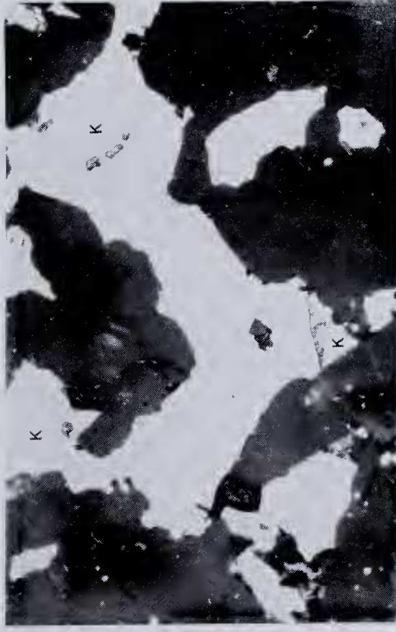
Figure 3.—Micrographs of the Yilmia I Meteorite. (a, top left) A metal rich region. The light phases are taenite and kamacite. Only two grains of sulphides are visible in this field. Width of field 2.2 mm. (b, top right) A sulphide rich region. The light areas are mainly troilite, alabandite, and daubréelite, with some schreibersite and a few metallic grains at the right hand edge. Oldhamite is present in some of the dark pits. Width of field 2.2 mm. (c, lower left) Alabandite altering along cracks to an oxide phase. The white area is troilite. Width of field 140 \mu . (d) Large schreibersite complex (white areas). Width of field 560 \mu . Kamacite grains marked K.
